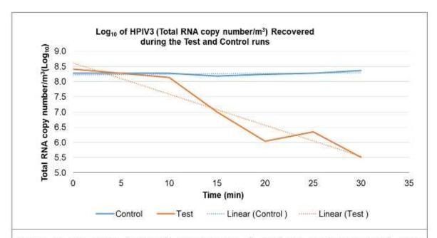
Figure 5.1. The effect of operating the Novaerus air purifier on aerosolised HPIV3. Lines represent the mean values obtained at each time point for control (blue) and test (orange) runs.
